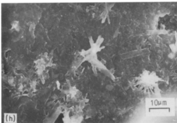
Figure 11 Scanning electron micrographs of a 280 μm fibre: (a and b) HTT = 220^{\circ}\text{C} , transverse section; (c) HTT = 220^{\circ}\text{C} , longitudinal section; (d) HTT = 220^{\circ}\text{C} , transverse section. SEMs of a 145 μm fibre: (e and f) HTT = 220^{\circ}\text{C} , longitudinal section; (g) HTT = 70^{\circ}\text{C} , transverse section; (h) 1.3 mm rolled sheet, transverse section.
